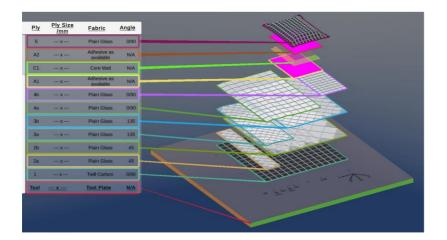
Composite parts, like fibre reinforced plastics, are manufactured from layers of material. Automating the process is capital-intensive and expensive. Operators manufacturing by hand leads to higher variability, more inspection and potentially more scrap.
